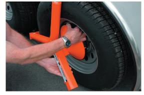
4. Insert the telescoping hook and snap the lock into the nearest hole.
